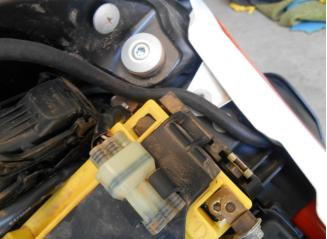
• Loop the breather line as indicated and cable tie in place and route down beside the battery to the rear of the LH crank cover.
