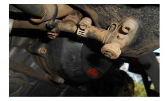
• Connect the LH & RH fuel lines to the rear Safari tanks with the 'T' connector on the LH side near the rear suspension shock absorber and cable tie in place.
