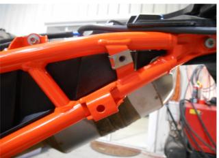
3. Install 2 captive nuts in locations 2 & 3 on the LH side (right hand side shown in photo) ready to install the tank.
