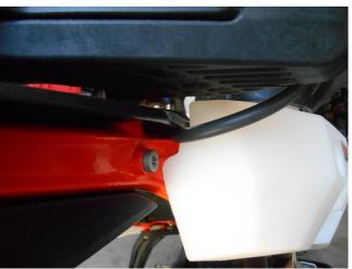
Route the longer length of breather line along the inner RH side of the motorcycle frame to the battery location.
